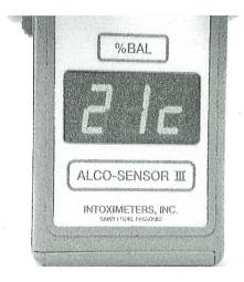
If the displayed temperature is below 15° C the unit may be warmed in a shirt pocket or similar manner. If the temperature is above 36° C, it will take time for the instrument interior to cool off. Keep it out of hot cars!
